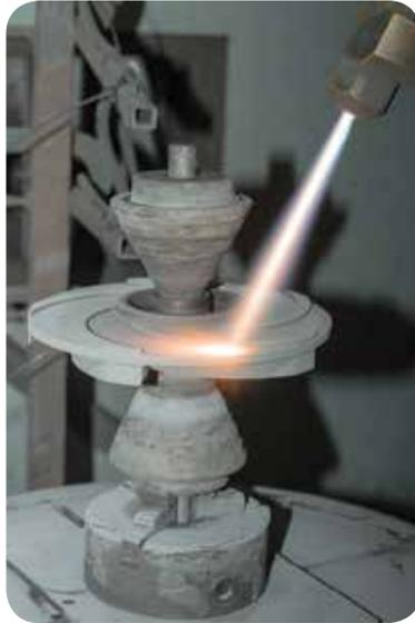
The HVOF coatings of today are successfully applied to a variety of substrates and typically exhibit higher densities, typical bond strengths greater than 80 MPa and low decarburisation levels.
