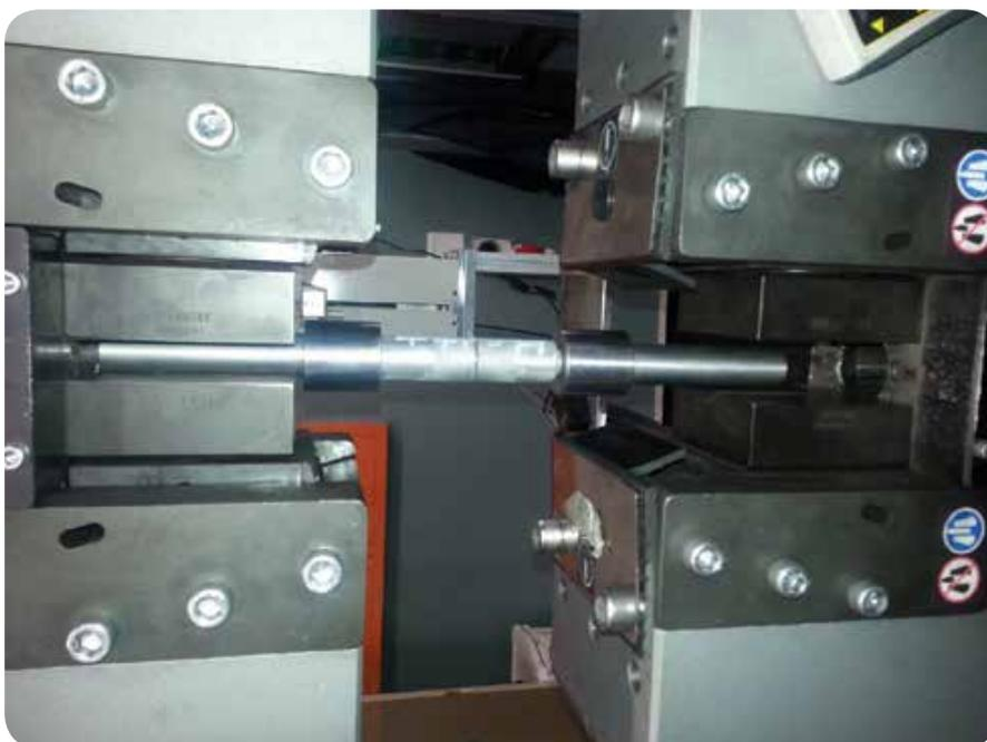
Adhesion tests in accordance with EN 582/ASTM C63 (above), along with the micro indentation tests are critical in defining coating quality.
