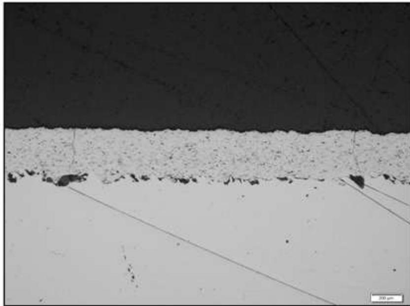
**Figure 4: Example of a poor coating with cracks and grit entrapment**
