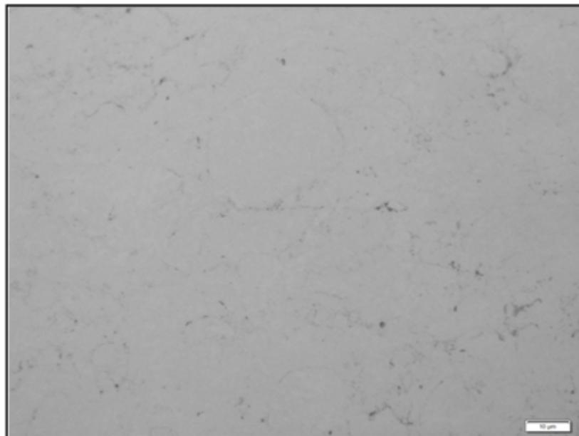
**Figure 10: Coating micrograph with low porosity and no defects**
