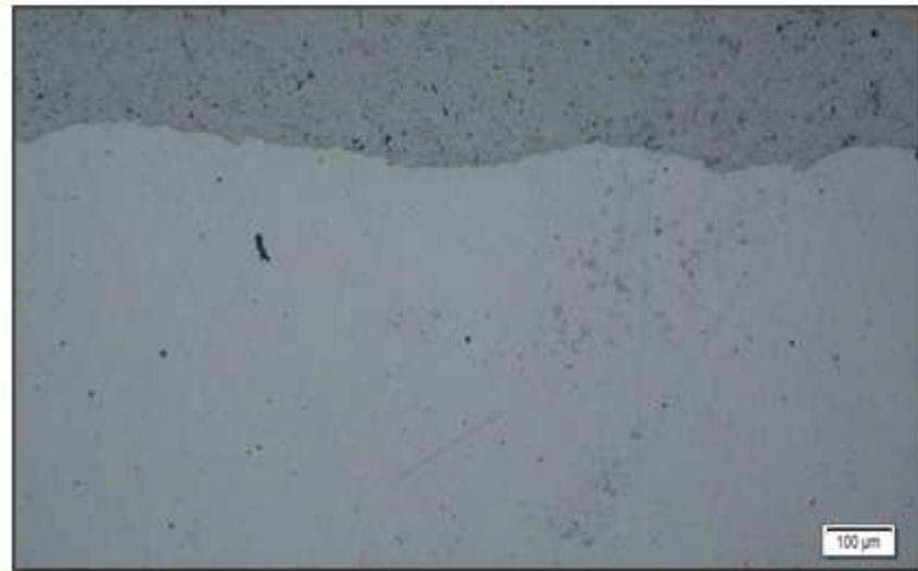
**Figure 9: Coating micrograph with no grit entrapment and low porosity**
