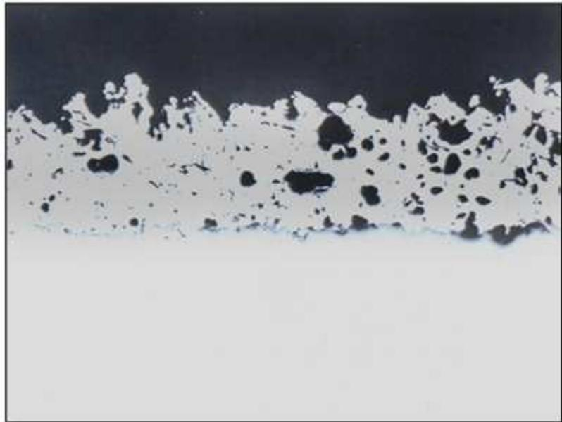
**Figure 6: High porosity in thermal coating**
