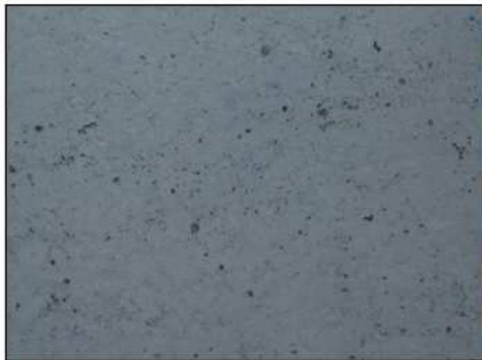
**Figure 8: Thermal spray coating micrograph with no defects and minimal porosity**
