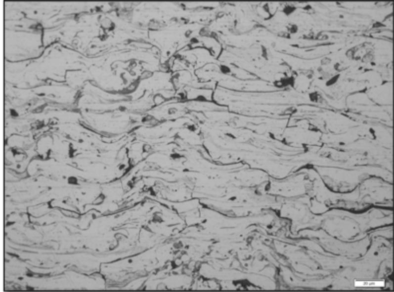
**Figure 5: Oxides in the coating**
