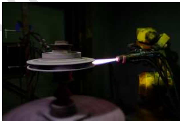
Figure 1: Pump impeller sprayed with the HVOF process
