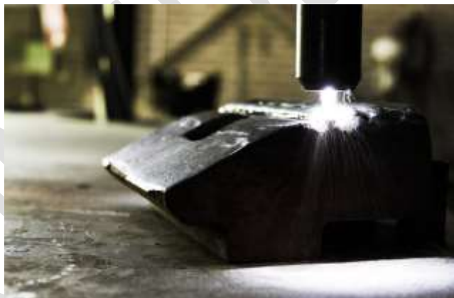
Figure 2: Plasma Transferred Arc (PTA) welding process
