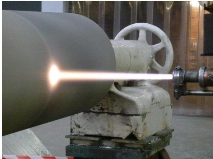
*Figure 3: Hydraulic Rod being thermally sprayed*
