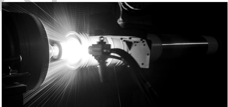
Figure 2: Arc Spray Process
