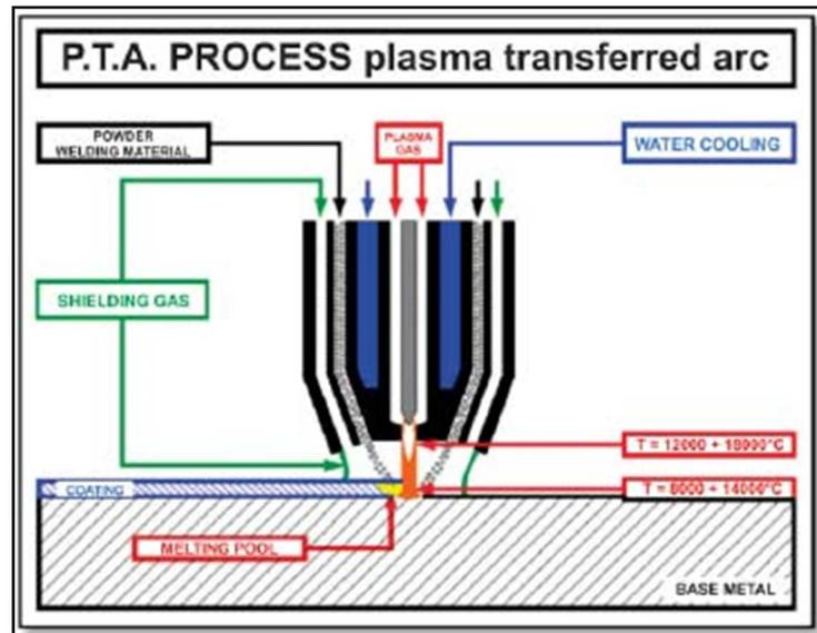
Figure 1: Schematic of the PTA process
