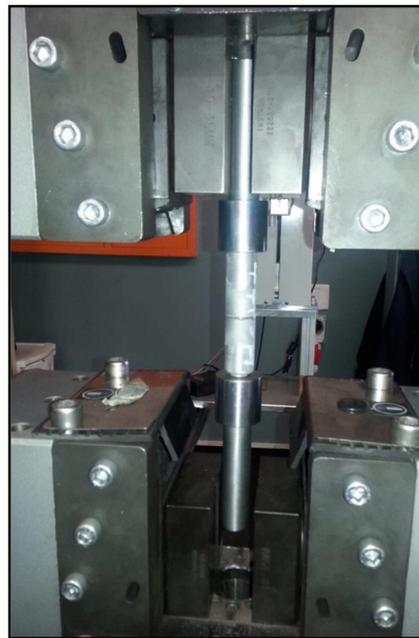
**Figure 1: Adhesion samples in testing configuration**
