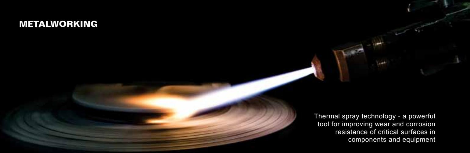
Thermal spray technology - a powerful tool for improving wear and corrosion resistance of critical surfaces in components and equipment
