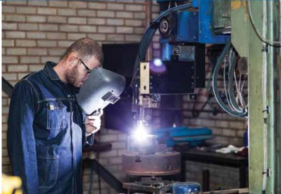
PTA welding is a hard-facing process that heats metals and merges them by means of arc constriction
