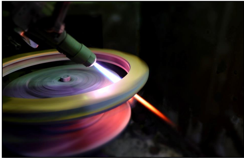
Figure 2: High Velocity Oxy-Fuel (HVOF) thermal spray process
