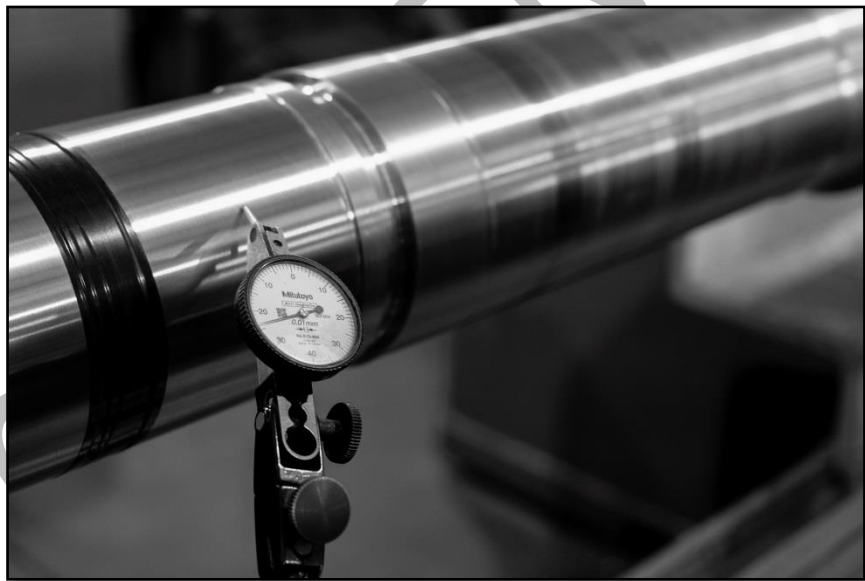
Figure 1: Shaft after thermal spray and grinding
