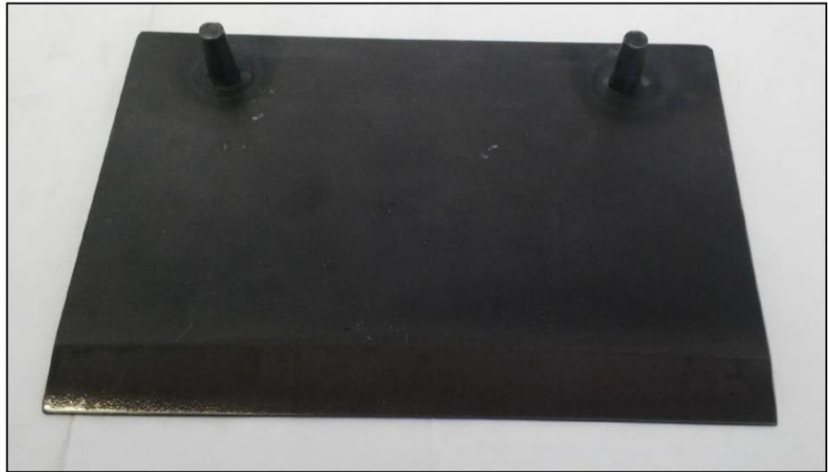
**Figure 2: Coated Transfer plate after 4 weeks service**
