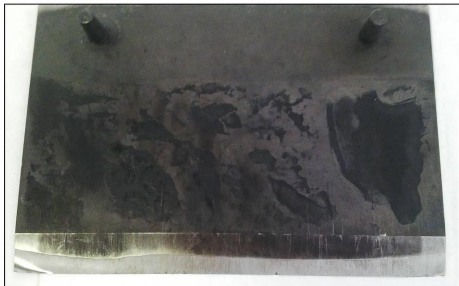
**Figure 1: Uncoated Transfer plate after 5 days in service**
