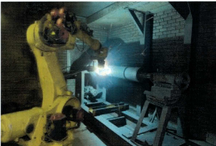
THERMAL SPRAYING Thermal spraying is defined as a group of coating processes in which finely divided feed materials are melted and sprayed on to a surface
