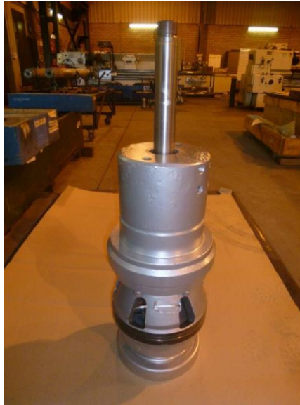
Figure 2: Inlet Sempel Valve
